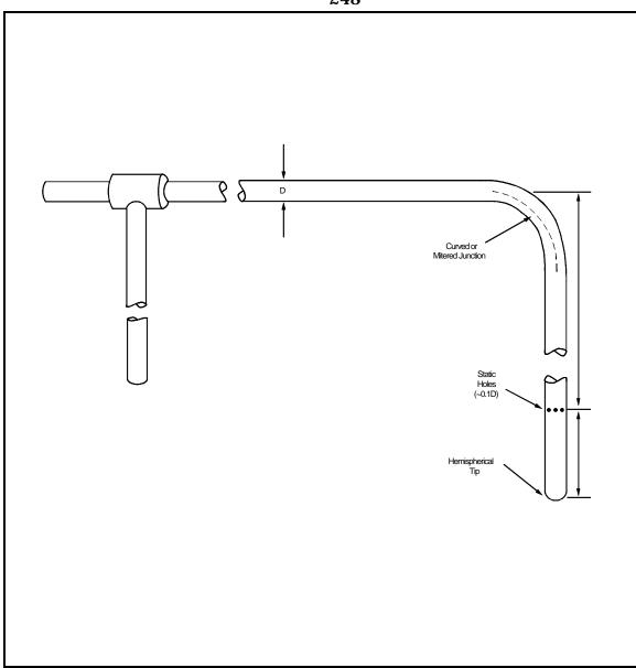
Figure 2-5. Standard pitot tube design specifications.
