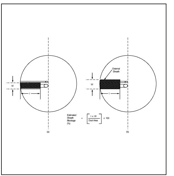
Figure 2-10. Projected-area models for typical pitot tube assemblie
