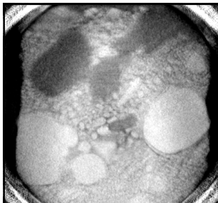
A conglomerate from Hot Ice #1 shows quartz and sandstone gravel cemented in a sand/ice matrix.
