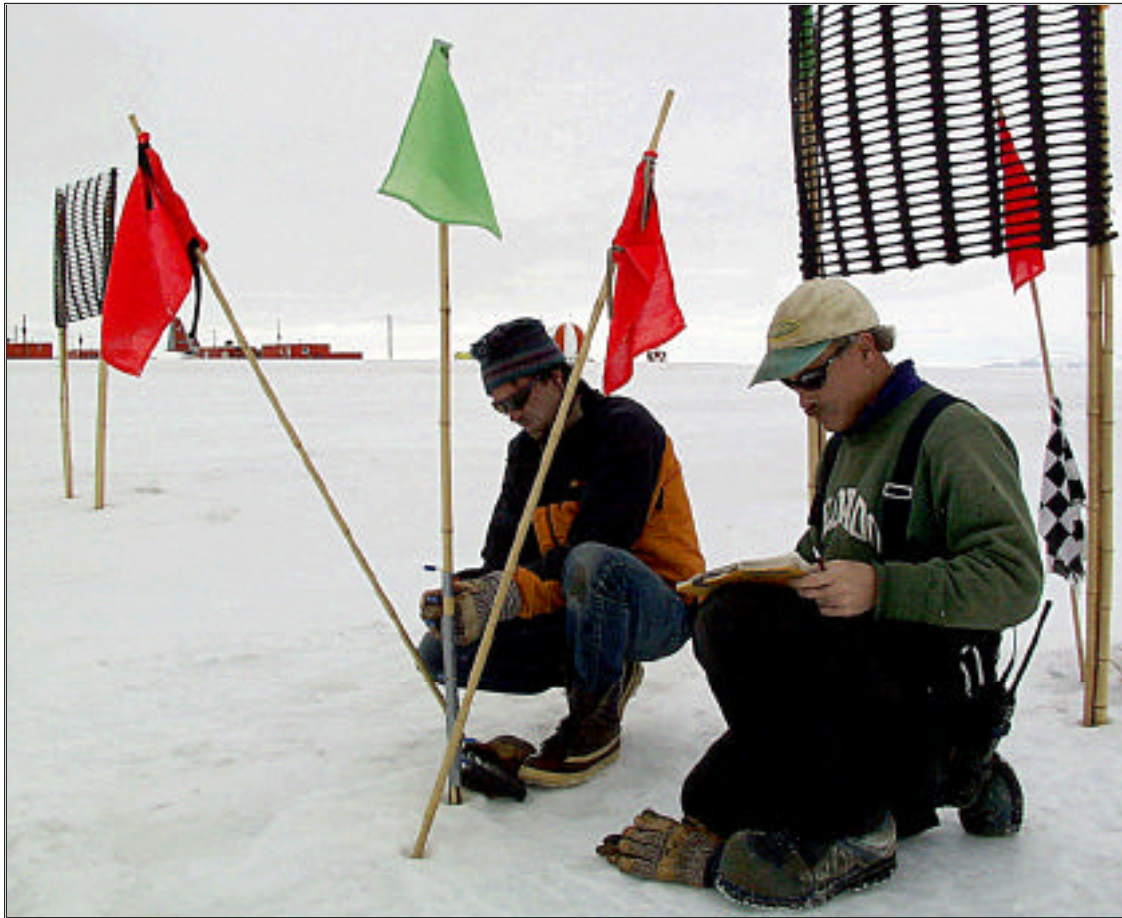
Surveyors Bob Champoux, left, and Jeff Scanniello take the season's last ice temperature readings at the ice runway. "The ice deteriorates really, really fast when it gets warm," Scanniello said.
