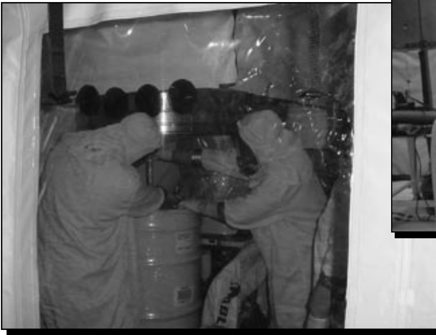
Drum load-out and size reduction operations at the TRU Waste Processing Facility
