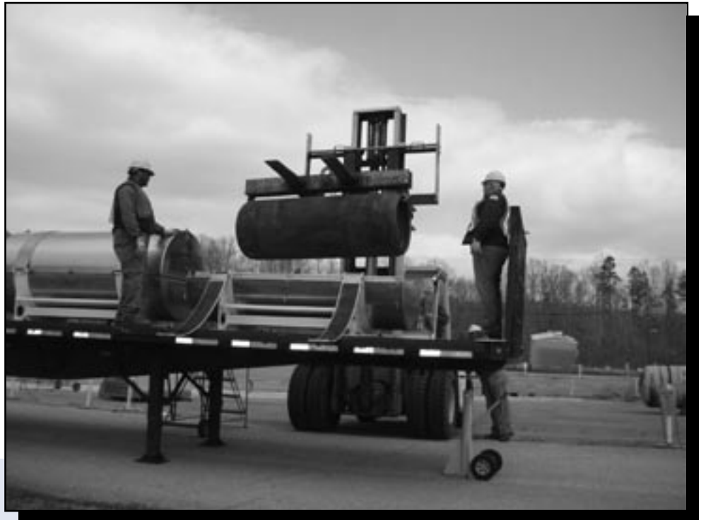
UF 6 cylinder being loaded for transport
