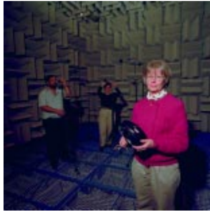
Figure 11. This fan, typical of space experiment payload noise sources, provides ventilation for a rack that houses a number of experiments.
