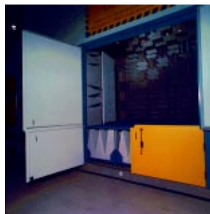
Figure 3. Test specimen access opening showing split door sections and wedge/floor modules on movable platforms.
