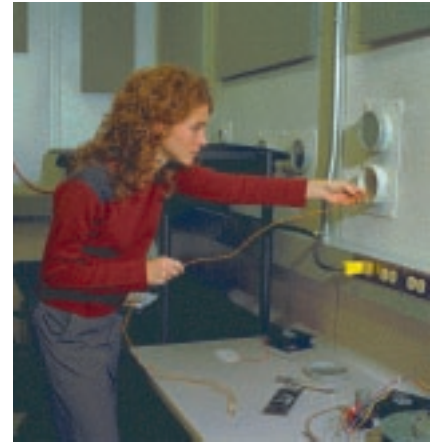
Figure 8. Test specimen service utilities are provided to the main test chamber interior by means of access sleeves with silencer plugs.
