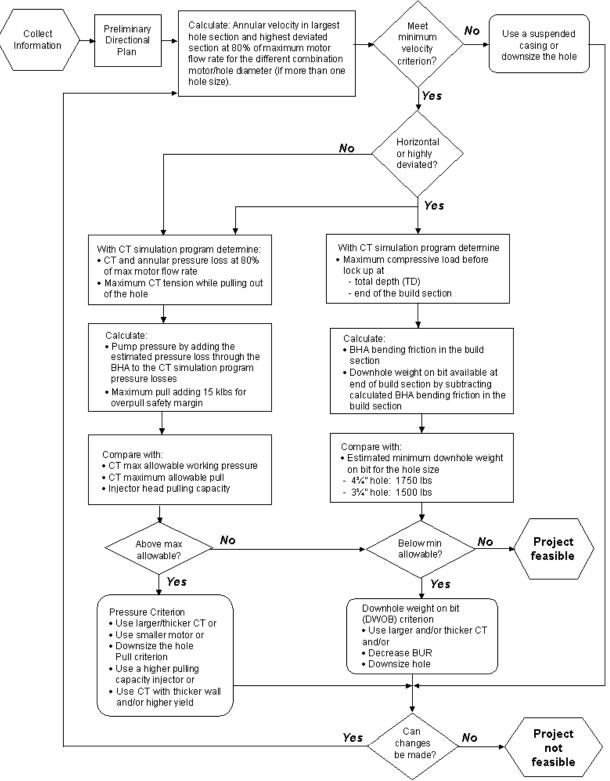
Figure 3: Example Procedure for Determining Feasibility of CTD
