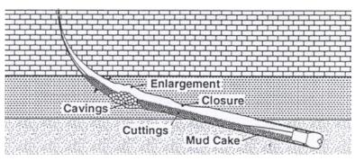
Figure 14. Hole Cleaning Problems
