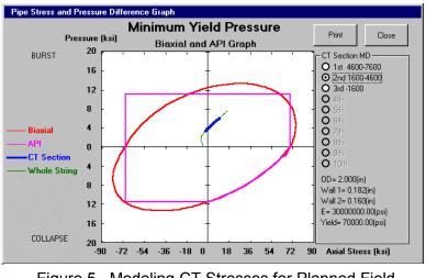
Figure 5. Modeling CT Stresses for Planned Field Operations (from MTI's CTPRO Model)
