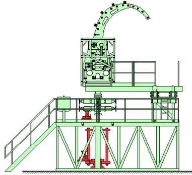
Figure 11. Multipurpose CT Support Structure
