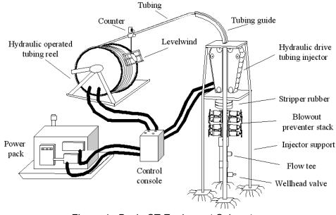
Figure 4. Basic CT Equipment Subsystems
