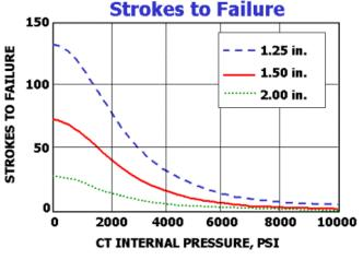
Figure 15. CT Life with Internal Pressure
