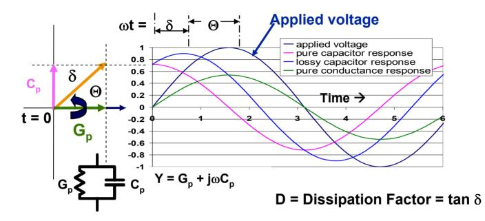
Ideal resistors have a response exactly in phase with the applied voltage (like the green curve).
