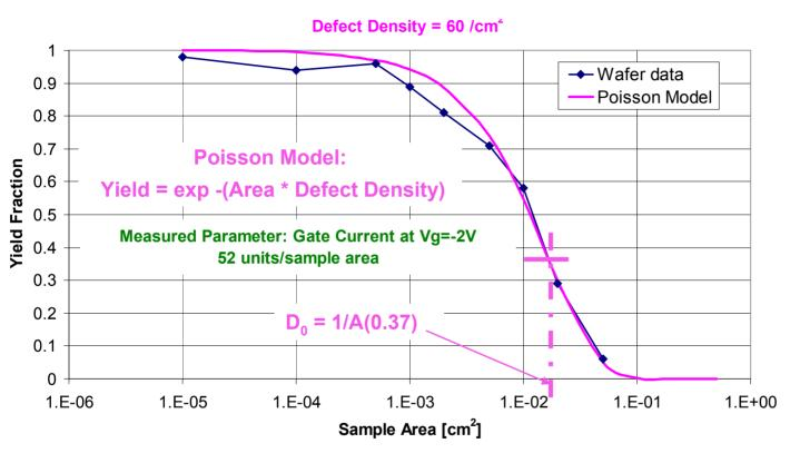
Assuming a good fit, defect density equals the inverse of the sample area for which the yield is 37%.
