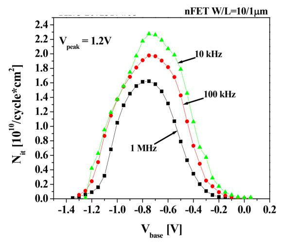
• Frequency dependence of interface state density is a characteristic of many high-k gate stacks.
