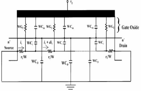
• This near-ultimate transmission line equivalent circuit was developed by Ahmed, et al.[1] It was used to show that channel lengths less than about 10  $\mu$ m are needed to assure proper response of devices with 2 nm gate oxides.
