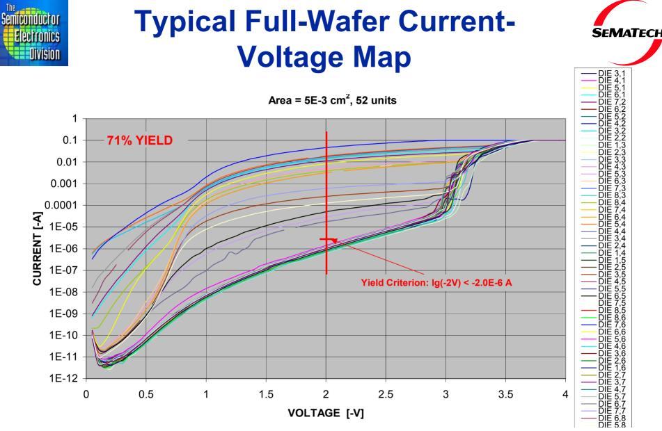
Yield criterion easily identified for a given wafer
