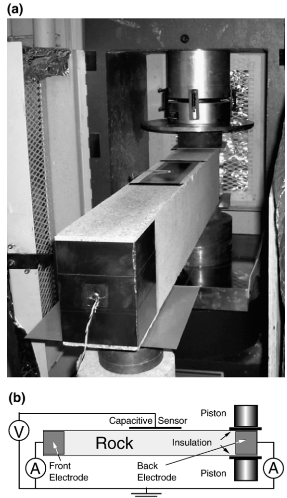
Fig. 1. (a): Granite slab placed in the press, ready for the uniaxial compression tests. The granite slab (1.2 m long, 10 \times 15 \text{ cm}^2 cross section) is fitted with two Cu electrodes ( 30 \times 15 \text{ cm}^2 ), one at the back end and one at the front end, plus a non-contact capacitive sensor for measuring the surface potential. The rock is insulated from the pistons and the press by 0.8 mm thick polyethylene sheets ( >10^{14} \Omega \text{ cm} ). (b): Block diagram of the electric circuit for allowing the self-generated currents to flow out of the stressed rock volume.
