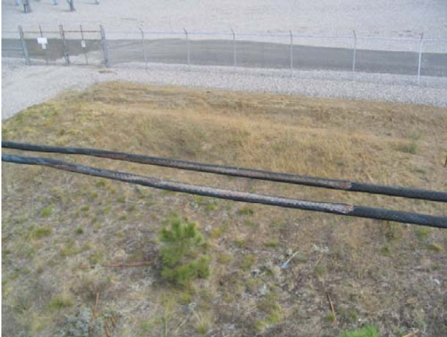
Close up picture of 13.8 Kv Kaiser power line (second conductor) showing paint transfer from left cross tube and indications of direction as cross tube moved across before tearing loose from aircraft.
