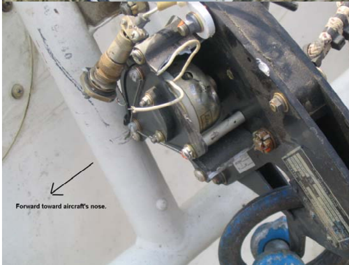
Aircraft's belly cargo hook. Pilot's electric release disabled due to contact with cargo suspension frame. Solenoid dents due to blue clevis bolt contact.
