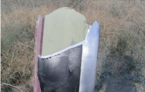
Photo of red M/R blade showing where blade wrapped around pole prior to braking.
