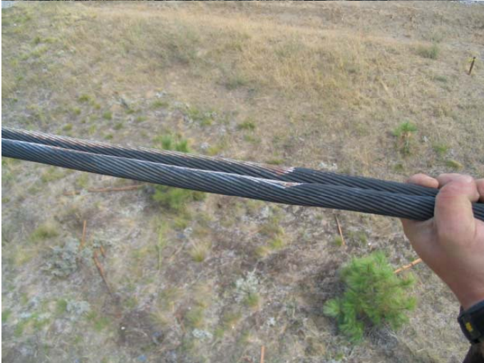
Picture of 13.8 Kv Kaiser power line (second conductor) shows paint transfer from left cross tube and indications of direction as cross tube moved across before tearing loose from aircraft.
