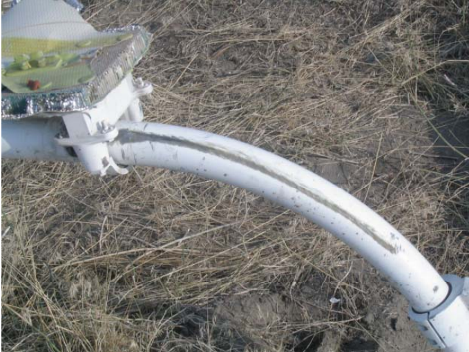
Left front cross tube scuffing is where landing gear caught on second conductor of 13.8 Kv Kaiser Feeder power line.
