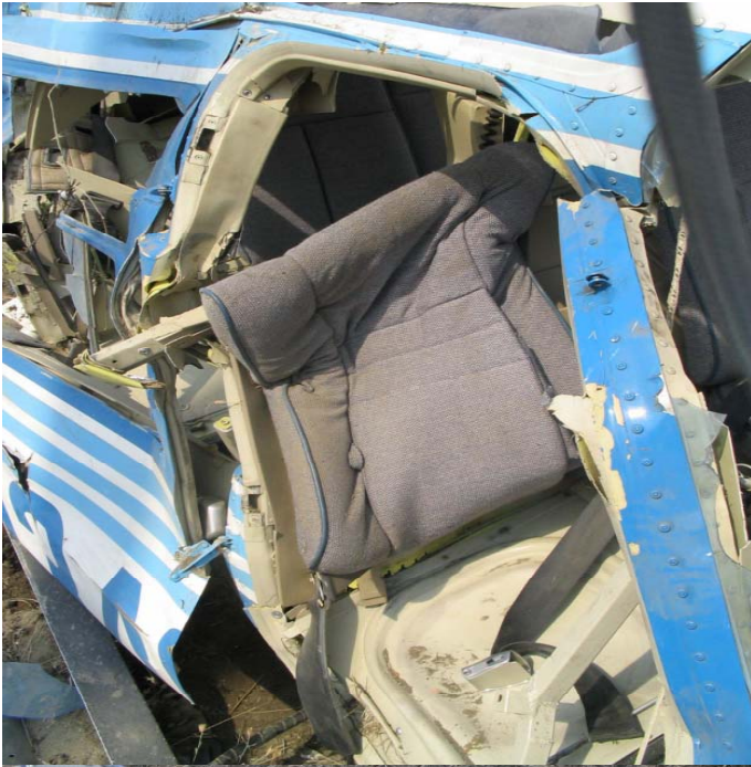
Right side close up shows extent of upper cabin crushing exposing pilot seat to ground impact.
