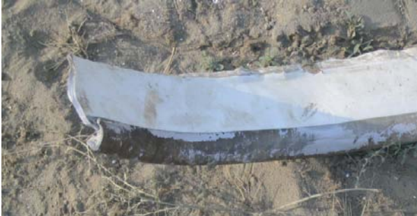
Photo of red M/R blade with creosote transfer from pole strike.
