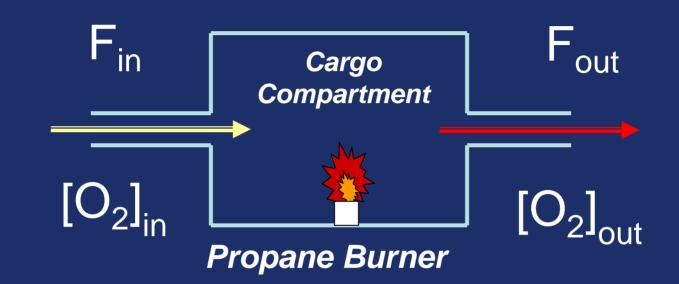
MASS BALANCE:  $\rho F_{in} = \rho F_{out} = \rho F$ SPECIES BALANCE:  $[O_2]_{in} - [O_2]_{out} = \Delta[O_2] = \theta$
