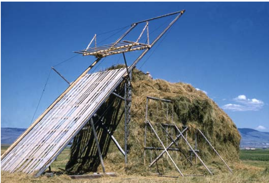
Figure 2.—Patented in 1909, the “Sunny Slope Slide Stacker,” commonly known as the “beaverslide,” remained popular until the 1990s, when it was largely displaced by mechanized equipment for producing large round bales of hay.
