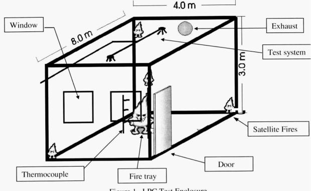
Figure 1. LPC Test Enclosure.
