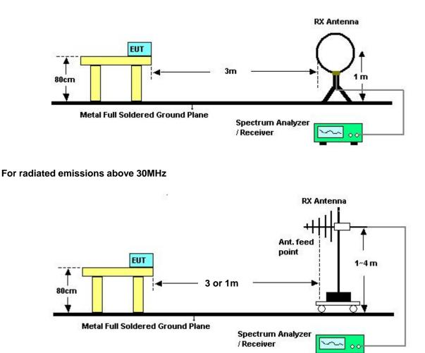
Above 10 GHz shall be extrapolated to the specified distance using an extrapolation factor of 20 dB/decade form 3m to 1m.
