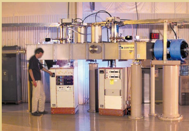
Livermore's Center for Accelerator Mass Spectrometry has developed specialized spectrometers for tritium (photo at left), heavy isotopes such as plutonium (photo at right), and carbon-14 (see p. 12), in addition to its large, multipurpose machine.
