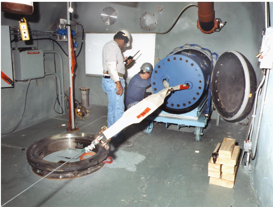
The steel vessel is pulled through the entryway into the experimental alcove.
