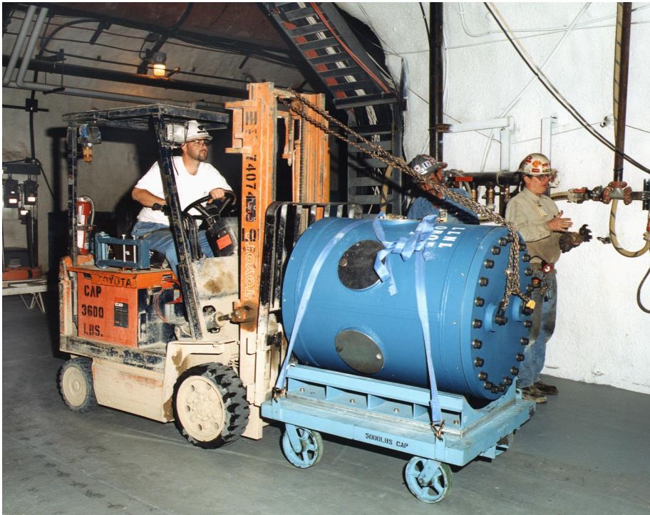
Once lowered downhole, a confinement vessel for the Oboe test series is transported to the experimental alcove. The vessel is designed to confine the gases and radioactive debris generated by a typical experiment.
