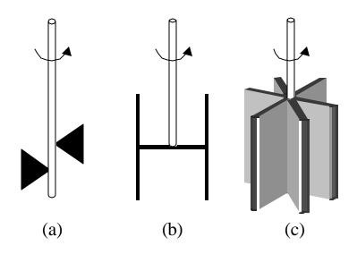
Figure 10 Various vane geometries used in concrete rheometers: (a) two-point test or Tattersall, (b) IBB, (c) BML.
