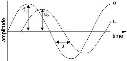
Figure 3 Sinusoidal wave forms for stress and strain functions.
