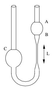
Figure 5 Ostwald type capillary viscometer. A and B are timing marks, C is a filling mark.
