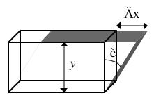
Figure 1 Shear strain schematic.
