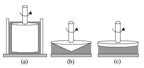
**Figure 8** Schematic diagram of basic tool geometries for the rotational rheometer: (a) concentric cylinder, (b) cone and plate, (c) parallel plate.
