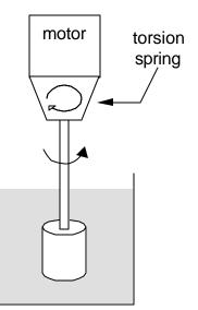
Figure 7 Schematic diagram of a Brookfield-type viscometer.
