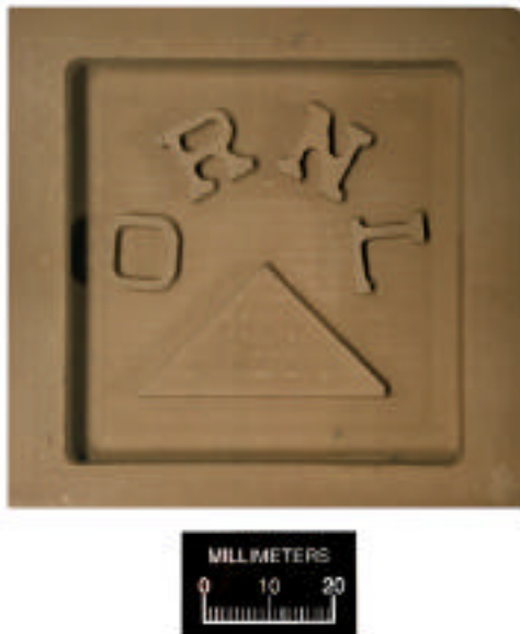
Figure 11. Gelcast silicon nitride can be easily machined in the green state and then fired to full density. Machining was accomplished on a computer controlled three-axis milling machine. (Techno/Isel Series Three CAM Production Center, New Hyde Park, NY)
