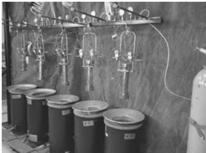
Using a continual shrinking bed counter current reactor, designed by NREL researchers, lignocellulosic biomass is totally hydrolyzed, using very dilute acid, for ethanol production.
