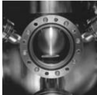
An NREL customized chamber demonstrated a pulsed laser deposition system where extremely high quality films of HTS are created.
