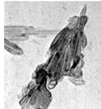
Carbon nanotubes hold hydrogen on their surface by adsorption and also within the tube structures. This has potential to significantly increase the amount of hydrogen contained over traditional activated carbon materials.
