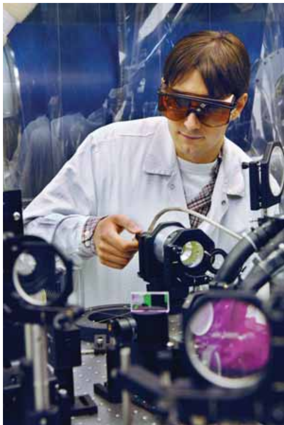
JENS SCHWARZ (1672) adjusts his group's newly patented Sandia optical tool that precorrects for laser distortions. (Photo by Randy Montoya)
