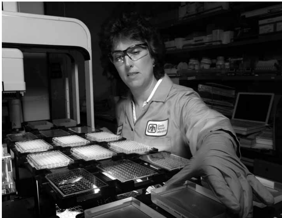
BIOCHEMIST JOANNE VOLPONI (8321) prepares samples of cellulase enzymes for activity assaying in a high-throughput, fluid-handling robotic system. Sandia is demonstrating various computational tools and enzyme engineering methods that can help process cellulosic biomass. (Photo by Randy Wong)
