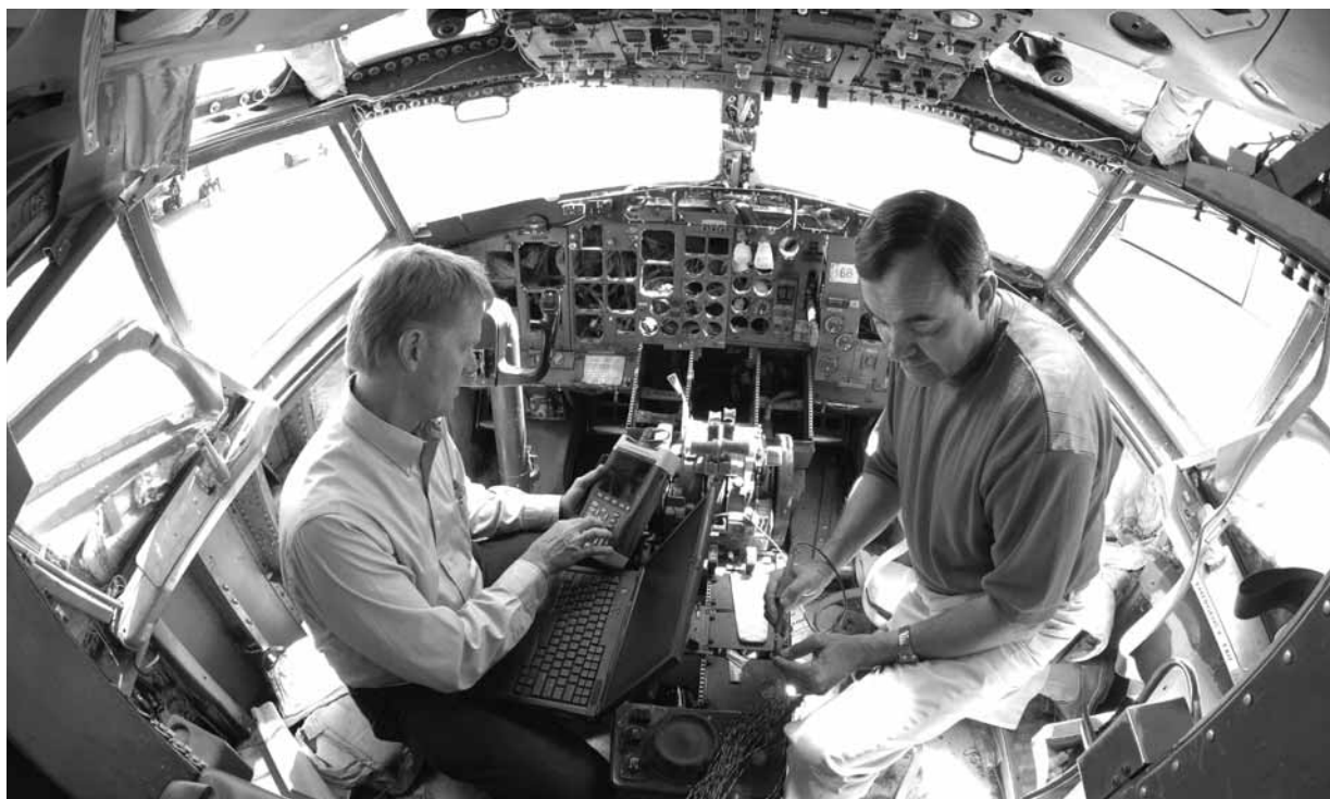
Mike Dinallo and Larry Schneider (left) prepare to employ the PASD diagnostic on a wiring bundle in the cockpit of a retired Boeing 737 at Sandia's FAA Airworthiness Assurance NDI Validation Center. (Photo by Randy Montoya)
