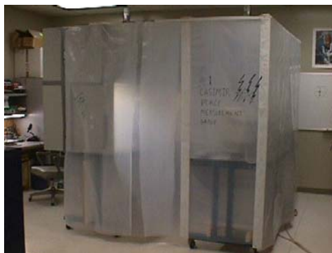
Figure 2.4: Clean room structure surrounding the AFM force measuring instrument. The structure contains two laminar flow HEPA hoods which maintain a positive pressure. The plastic walls stop about 1 inch above the ground to allow flow lines to remove dust from the cleanroom.
