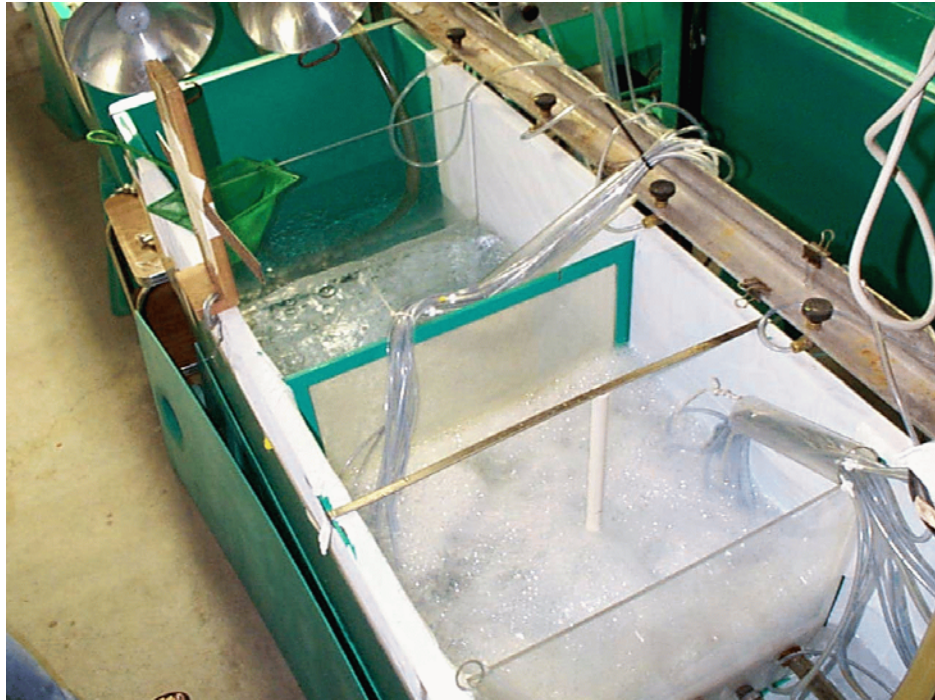
Fig. 2.1. Photo of observation tank showing (a) observation area lined by white plastic and (b) stress area with turbulence generated by aerators and water pumps.
