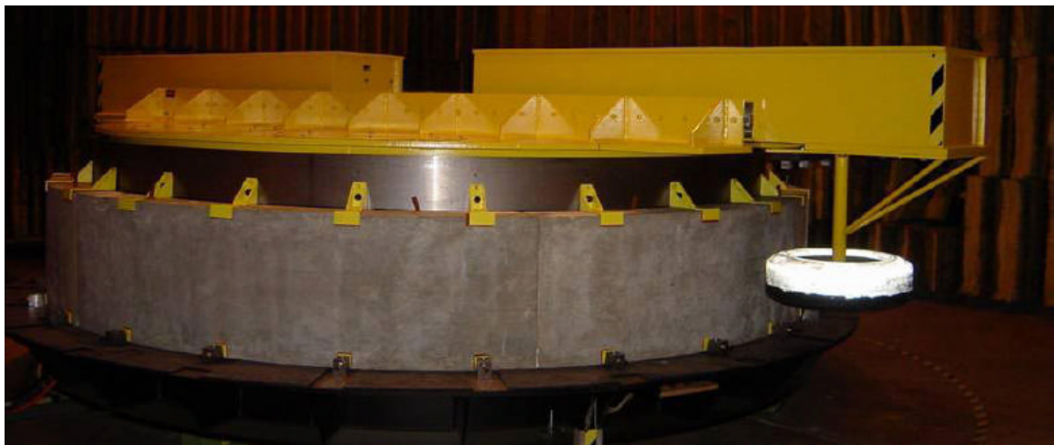
Figure 10.2 A closer view of the TPTA with the pavement sections
