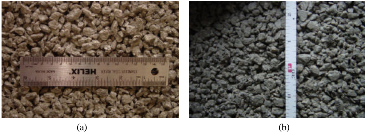
Figure 10.5 Surface appearances of EPC (a) 100% # 4 aggregates, and (b) 75% # 4, 25% # 8 aggregates
