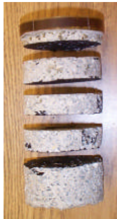
Figure 4.2 Sectioning the core for image analysis
