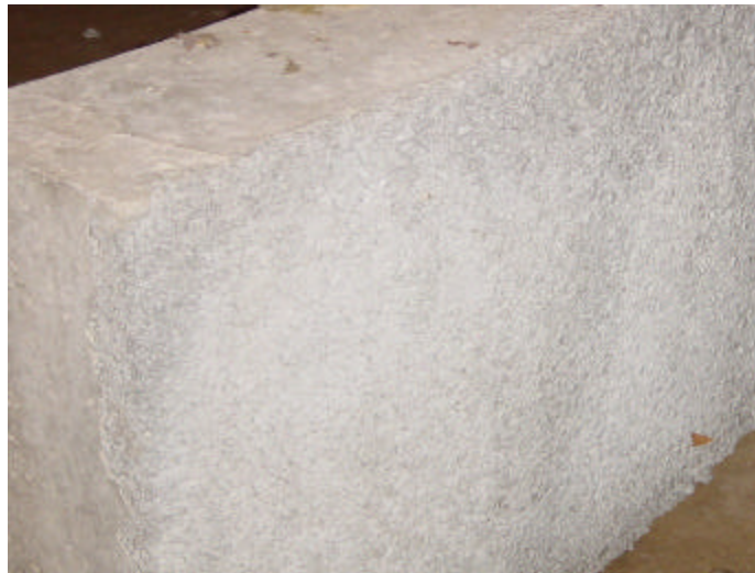
Figure 10.4 A closer look at an EPC specimen
