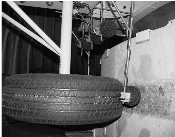
Figure 10.6 Five microphone array that travels with the tire
