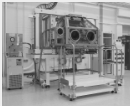
The LSG PDU system set up and ready for ISS science and engineering evaluations.
