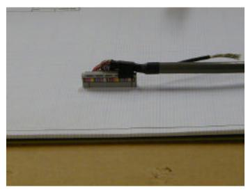
Cables use tubing threaded under cable strain relief to hold exposed cable in place
