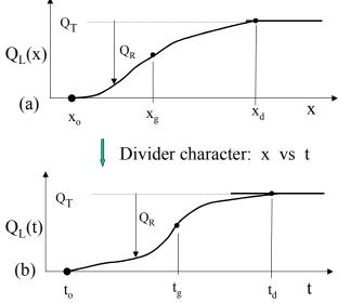
**Figure 3.** Divided flows as function of flow diverter position or time.
