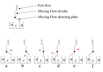
**Figure 7.** Option II - A translating diverter value with a rotating flow-directing device. Tanks are stationary.
