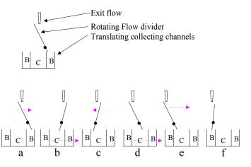
**Figure 8.** *Option III* – A rotating diverter valve with translating flow-directing channels.
