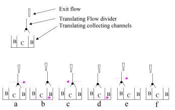
Figure 9 Option IV – A translating diverter valve with translating flow-directing channels.
