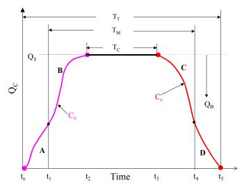
Figure 1. Liquid flow collected as function of time. For clarity, the constant collecting flow interval,  $T_c$ , has been compressed.
