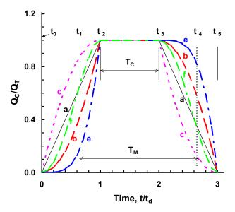
Figure 5. The collection flow as function of time for the six examples [Case (d) = Case (b)],  $T_M = t_d + T_C$ .
