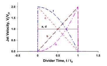
**Figure 4.** Jet velocity distribution as function of the diverter valve movement time. [Case (a) = Case (d)].
