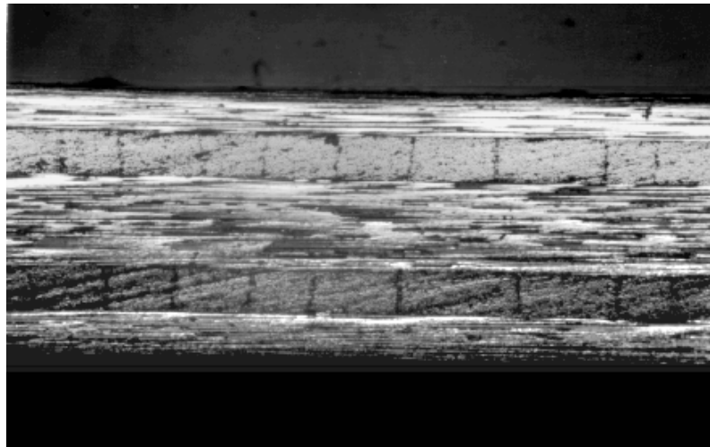
FIGURE 43. EVIDENCE OF 90° PLY MATRIX CRACKS IN [0/90/0] AND [0/90/0]_s LAMINATES OF AS4/3501-6 GRAPHITE-EPOXY COMPOSITE
