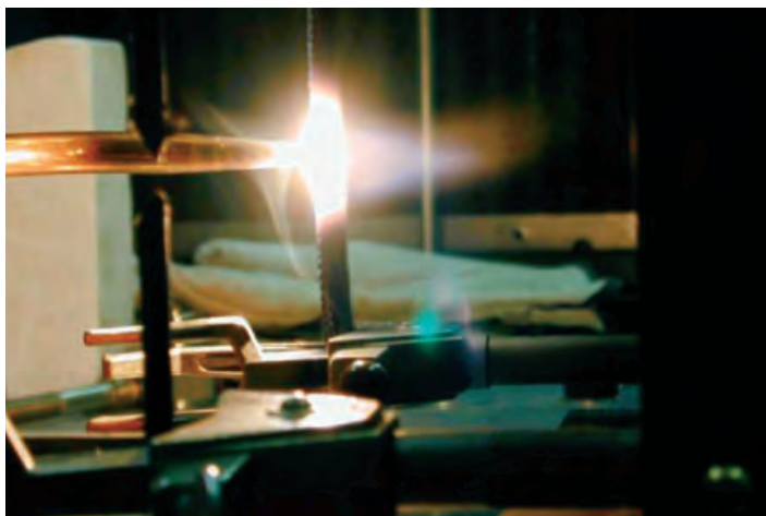
The carbon thermal barrier seal passes a torch test with flying colors.
