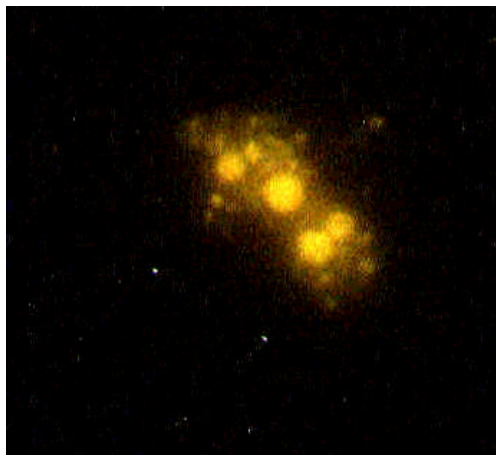
Plate 1. Cluster of oil droplet and bacteria under epifluorescence at a magnification of \times 400 , the biggest oil droplet diameter is 5 \mu\text{m}
