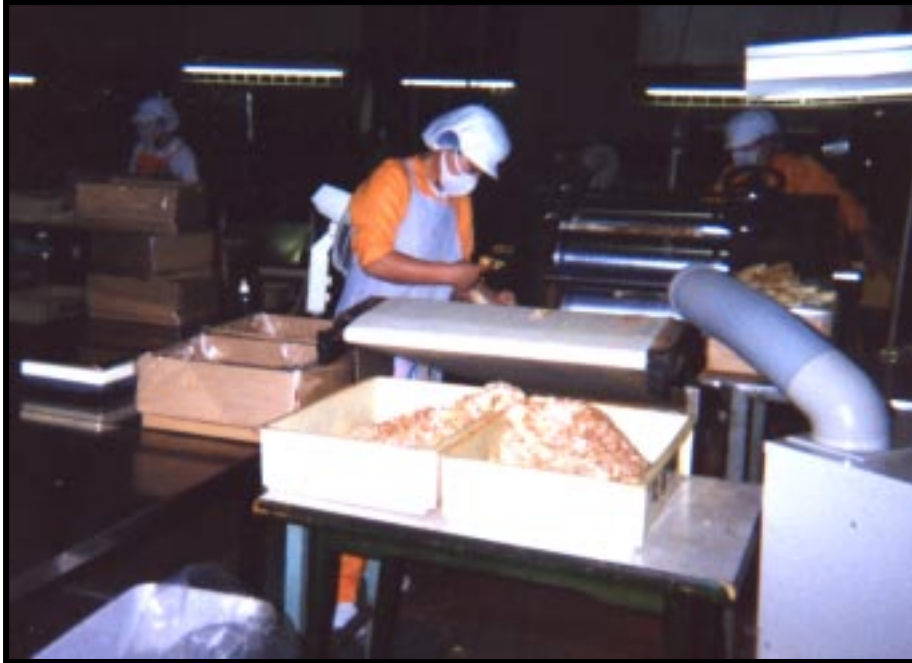
4-4 Tenderizing dried fish by smashing the fish through rollers to break down fibers.
