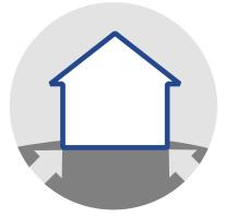
In climates with mild winters, slab insulation in a typical 1,800 square-foot home would save \$50 to \$60 annually. R-10 slab insulation for an 1,800 square-foot home would typically cost \$300 to \$600 to install. Thus, the insulation would pay for itself in 5 to 10 years.
