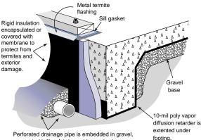
Perforated drainage pipe is embedded in gravel, covered with filter fabric, and located at lower perimeter of foundation footing to provide drainage.
