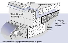
Perforated drainage pipe is embedded in gravel, covered with filter fabric, and located at lower perimeter of foundation footing to provide drainage.
