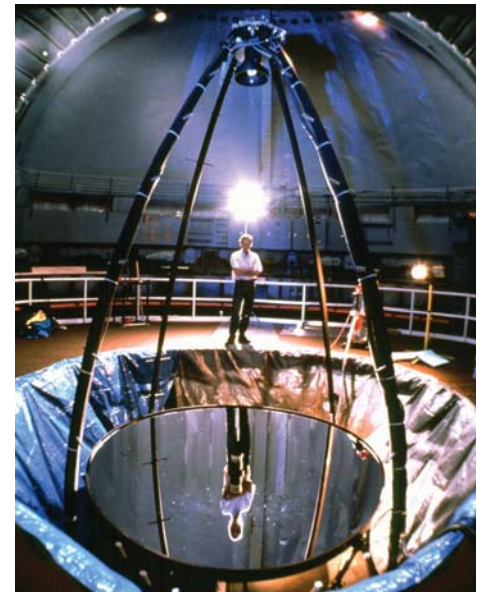
Figure 2. The 3.0 m NASA-LMT inside the NODO dome. The mirror is rotating at 10 rpm and the mercury (Hg) is fully oxidized.
