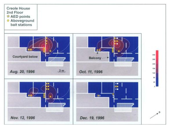
Figure 6. Spatial depiction of C. formosanus feeding activity in the wooden floor of the second floor of the Creole House during the baiting period. Stars give positions from which acoustic emission counts were taken and circles represent above-ground bait stations. Symbol colors depict the presence (yellow) and absence (white) of termite activity. Color bar and associated numbers represent AED count per minute.
