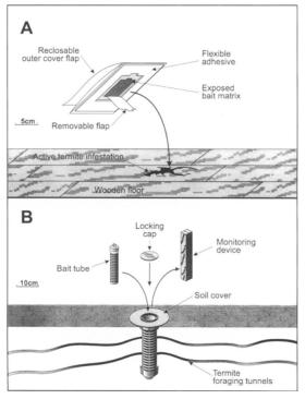
Figure 3. Above-ground bait stations consisting of a flexible laminated pouch containing 15g of 0.5% hexaflumuron bait (A) were placed directly over active infestations of C. formosanus in the wooden floors of the Bust Gallery of the Presbytere and the second floor of the Creole House. In-ground (Sentricon) stations were placed in the soil of the Creole House courtyard to detect termites and deliver hexaflumuron baits (B).
