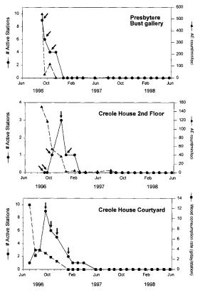
Figure 5. Coptotermes formosanus activities quantified by the number of both monitoring and baiting stations with live termites (circles with solid lines), acoustic emission counts (triangles with dashed line), and wood consumption rates (squares with dashed line) in the Bust Gallery of the Presbytere and the Creole House of the Cabildo. Arrows depict applications of baits containing 0.5% hexaflumuron.
