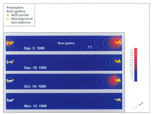
Figure 4. Spatial depiction of C. formosanus feeding activity in the wooden floor of the Bust Gallery of the Presbytere during the baiting period. Stars give positions from which acoustic emission counts were taken and circles represent above-ground bait stations. Symbol colors depict the presence (yellow) and absence (white) of termite activity. Color bar and associated numbers represent AED count per minute.
