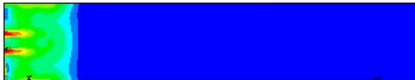
von Mises stress 700 nanosecs after pulse
