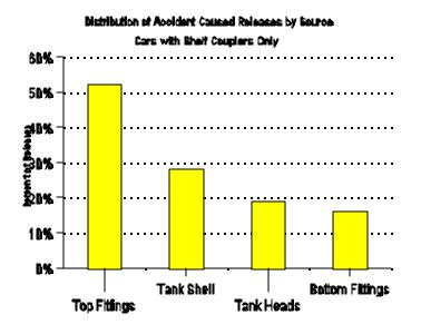
Although the distribution of accident-caused releases shows that top fittings account for more than 50 percent, the average percent of lading lost is about 1/3 of that from other sources. The data suggests that the quantity of product released from damaged fittings is less than that from a head or shell puncture or sheared-off bottom outlet. The following chart shows the average percent of lading lost in accident-caused releases by source.
