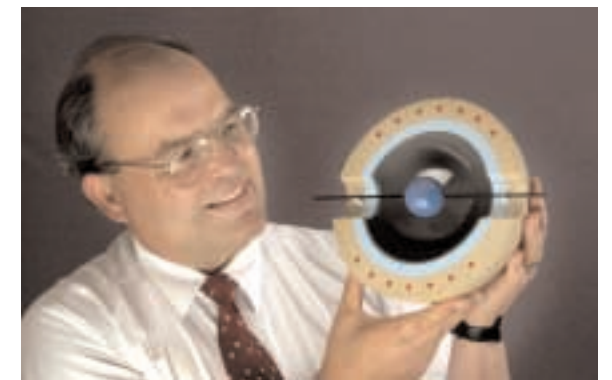
FISSION BATTERY? — Gary Rochau, Manager of Modeling and Analysis Dept. 6415, holds a cutaway model of a magnetically insulated fission electric cell. Gary’s group is planning a proof-of-principle experiment to demonstrate that electricity can be provided directly from fission, without boiling water.
