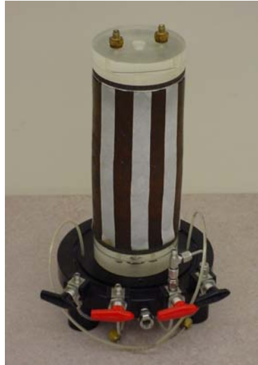
Figure 3.9. Triaxial sample of RAP-soil mixture on base pedestal
