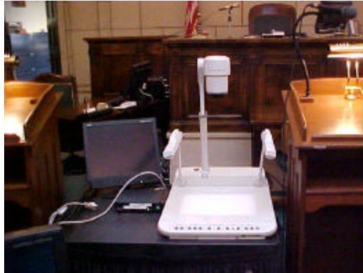
The Evidence Presentation Cart: Includes the document camera, monitor and one VGA connection for a laptop.
