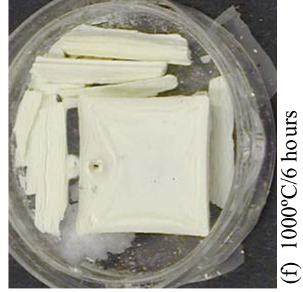
Figure 1. Appearance of tantalum Alloy T-222 specimens tested in flowing air at various times and temperatures.
