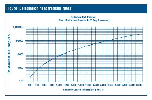
The biggest radiant energy loss in furnace operations is caused by doors remaining open longer than necessary, or doors left partially open to accommodate a load that is too large for the furnace. Furnace openings not only waste energy through radiation losses, they also allow ambient air to enter the furnace or hot furnace gases to escape if the furnace pressure is not controlled (see the tip sheets titled *Reduce Air Infiltration in Furnaces; Furnace Pressure Controllers*).
