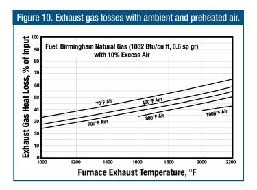
Waste heat recovery. Reducing exhaust losses should always be the first step in a well-planned energy conservation program. Once that goal has been met, consider the next level – waste heat recovery. Waste heat recovery elevates furnace efficiency to higher levels, because it extracts energy from the exhaust gases and recycles it to the process. Significant efficiency improvements can be made even on furnaces that operate
