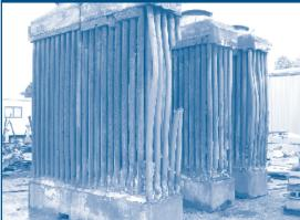
mixture after the liquid evaporates. Slag is the residue formed by oxidation at the surface of molten metals, which can also adhere to heat transfer surfaces. These contaminants impede the efficient transfer of heat and reduce the efficiency of industrial heating systems.
