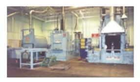
A quench furnace line for heat treating.
