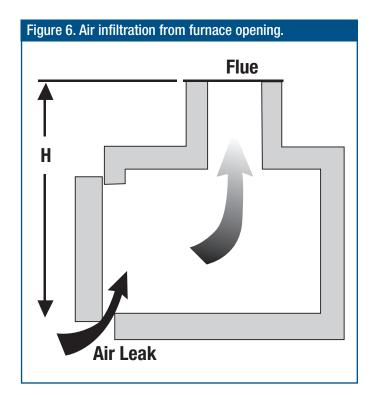
The bottom line is that to get the best possible energy efficiency from furnaces and ovens, reduce the amount of energy carried out by the exhaust and lost to heat storage, wall conduction, conveying and cooling systems and radiation.
