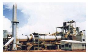
A rotary dryer for removal of free water.
