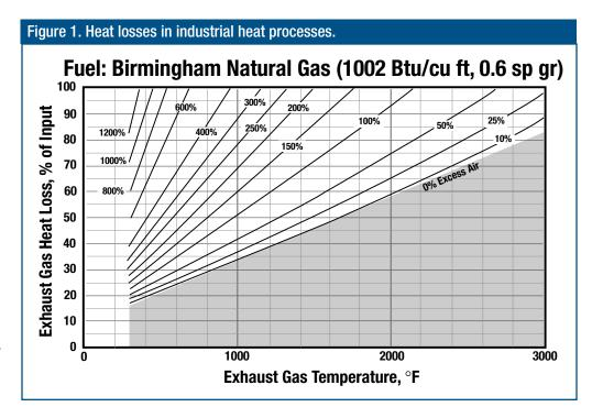
This makes it obvious that the temperature of a process, or more correctly, of its exhaust gases, is a major factor in its energy efficiency. The higher that temperature, the lower the efficiency.
