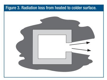
Anywhere or anytime there is an opening in the furnace enclosure, heat is lost by radiation, often at a rapid rate. These openings include the furnace flues and stacks themselves, as well as doors left partially open to accommodate oversized work in the furnace
