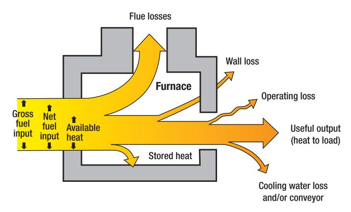
Figure 3. Energy loss diagram in a fuel-based process heating system.
