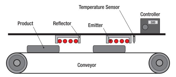
Figure 5. An electric infrared heating system.
