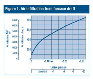
through the stack. This negative pressure causes ambient air to leak into the furnace.
