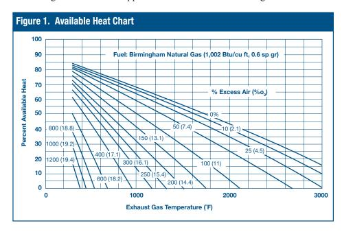
The amount of energy savings obtained by using load preheating is *higher* than the amount of actual heat transferred to the load. The "net" heat delivered to the load has to account for the efficiency of the furnace. Since the furnace efficiency is always less than 100%, the resulting energy savings exceed the energy picked up by the load. Load preheating can result in higher production from the same furnace.
