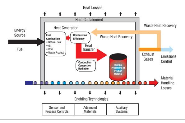
Figure 2. A fuel-based process heating system and opportunities for improvement.
