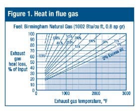
from the furnace via a flue or stack. At this point, these gases still hold considerable thermal energy. In many systems, this is the greatest single heat loss. The energy efficiency can often be increased by using waste heat gas recovery systems to capture and use some of the energy in the flue gas.
