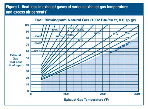
Before attempting to use energy from higher temperature flue gases in lower temperature processes, engineers should take the following technical issues into consideration:
