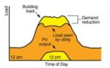
The correlation is high between commercial load (building) demand and solar availability. So PV provides power when needed, thus displacing peak energy and reducing demand.
