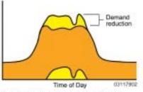
The Solar Load Controller (SLC) reduces the load when needed by acting on end-use settings or scheduling. Because of the naturally high correlation between PV and load, the end-use inconvenience is minimal compared to the demand reduction enhancement.
