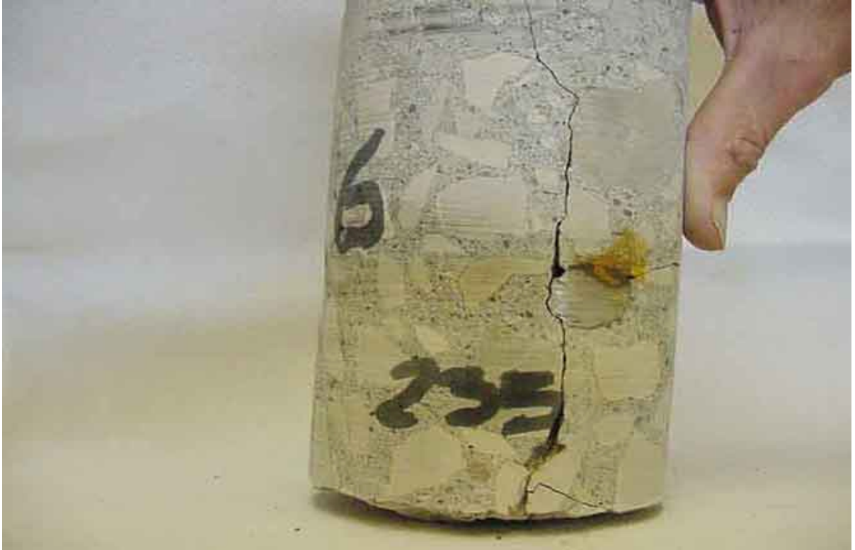
Core showing crack propagating from corroded reinforcing steel in parent concrete
