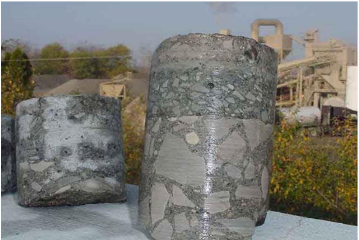
Core showing bond line
