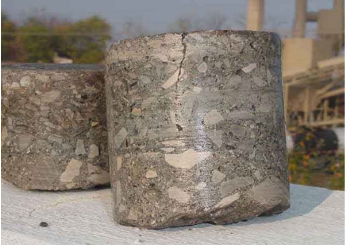
Crack extending part way through overlay
