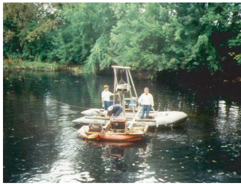
Figure 5.70 Shallow water vibratory core collection.
