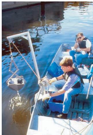
Figure 5.67 Winch with Ponar dredge.
