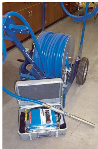
Figure 5.40 Grundfos Redi-Flo2 pump sampler with controller.
