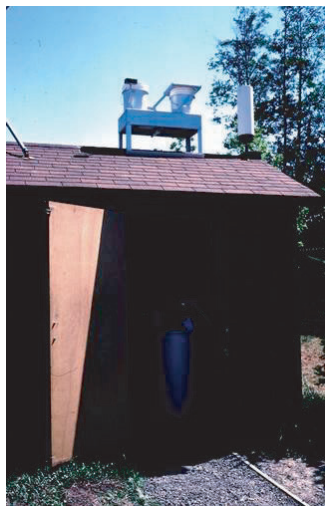
Figure 5.58 Wet-dry atmospheric deposition sampler in Bellevue, WA.
