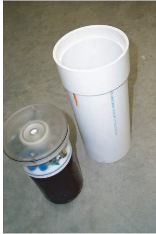
Figure 5.50 Prototype WI DNR/USGS automatic sheetflow sampler.
