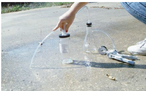
Figure 5.47 Sheetflow sampler operated by hand vacuum pump.
