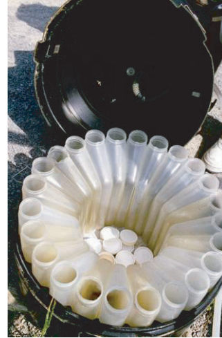
Figure 5.21 Discrete sample bottle base for ISCO automatic sampler.
