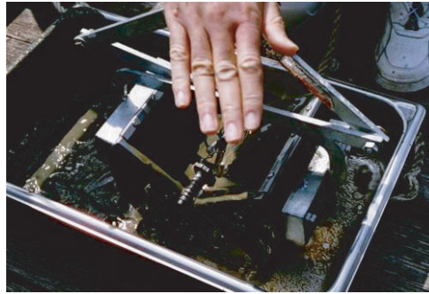
Figure 5.66- Emptying Ponar sample into stainless steel sample pan.
