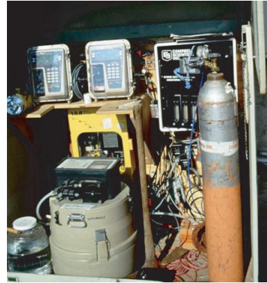
Figure 5.17 ISCO sampler used in instrument shelter with flow monitoring and telemetry equipment in Madison, WI.
