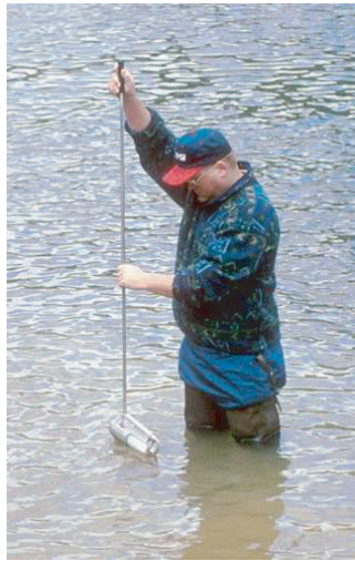
Figure 5.45 .Depth-integrated sediment sampler being readied for use.
