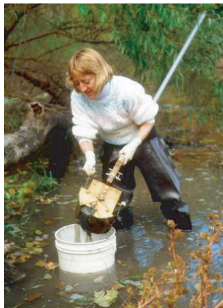
Figure 5.69 Collecting sediment with an Ekman dredge.
