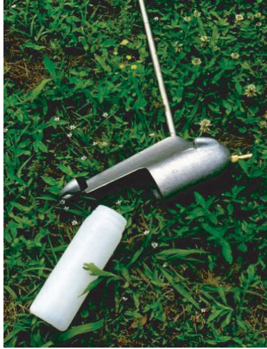
Figure 5.43 .Depth-integrated sediment sampler parts.
