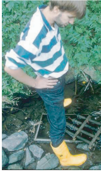
Figure 5.28 In-stream continuous probes at Dortmund, Germany, CSO monitoring site.
