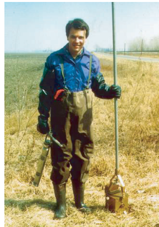
Figure 5.68 Hand-held corer and Ekman dredge.
