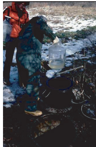
Figure 5.22 Composite sample bottle from Toronto snowmelt sampler.
