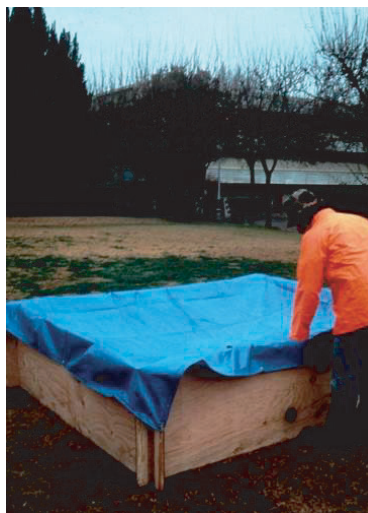
Figure 5.59 Large surface area used to capture sufficient rain for chemical analyses in early San Jose, CA, tests.
