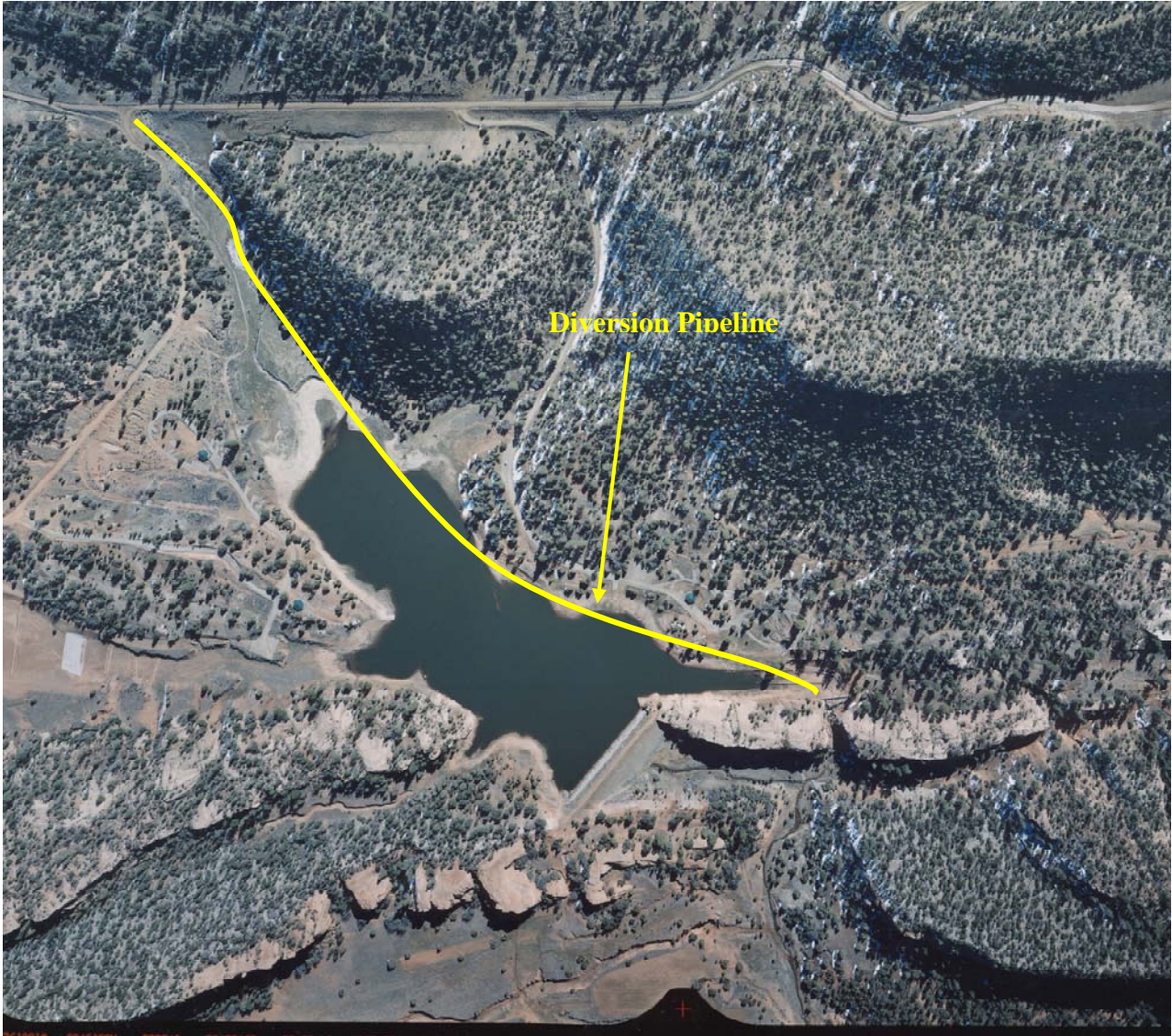
Figure 6. Proposed Stream Diversion Pipeline Route.
