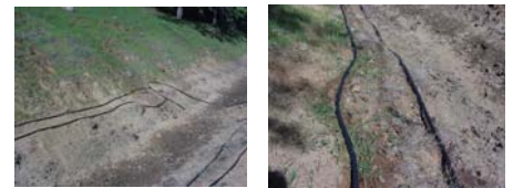
View of the soaker hose array used to apply acetic acid solutions to the plots.
