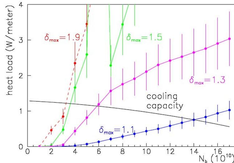
Simulated average LHC arc heat load and cooling capacity as a function of bunch population  $N_b$ , for various  $\delta_{max}$ . Other parameters are  $\epsilon_{max} = 262$  eV,  $R = 5\%$ ,  $Y = 5\%$ , and elastic electron reflection included. Average:  $l_{dip} = 3 \times 14.3$  m,  $l_{drift} = (3 \times 1.36 + 2.425)$  m,  $l_{quad} = 4.045$  m.
