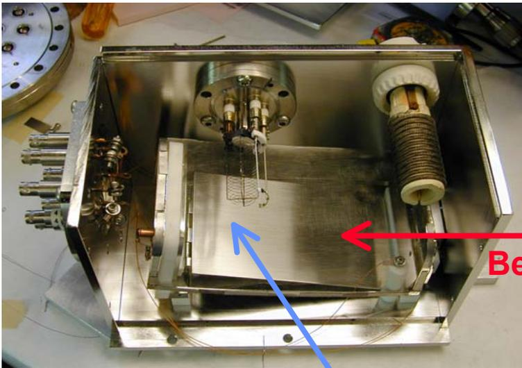
Target surface roughened by glass-bead blasting – grazing incidence ions now hit rims of craters.
