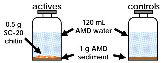
Figure 4. Schematic of the microcosm experiments.
