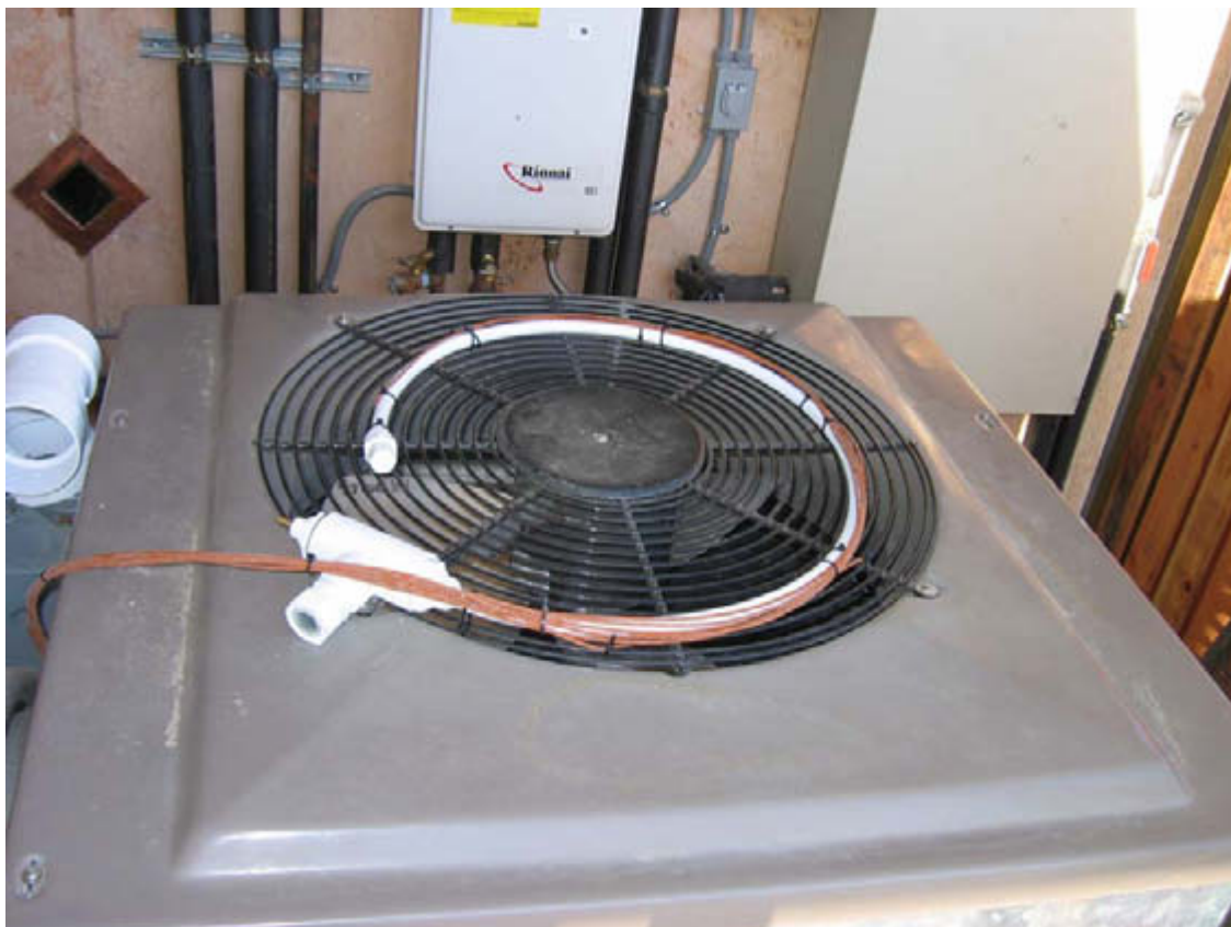
Figure 27. Thermocouple (brown wire) and sampling tube (white PVC shield plus white tube) installed at Freus exhaust grill. Vacuum pump housing shown on left (White PVC pipe fitting)
