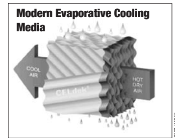
Figure A. Direct evaporative coolers use a fan to pull outside air through pads that are wet (left), filtering and cooling the air (right).
