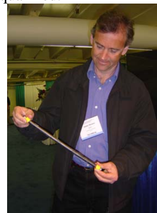
FIGURE 5: The head of the EMPA team from Switzerland, Gabor Kovacs, is holding an element of the dielectric EAP actuator. To drive their robotic arm 256 such elements were used in a protagonist-antagonist system
