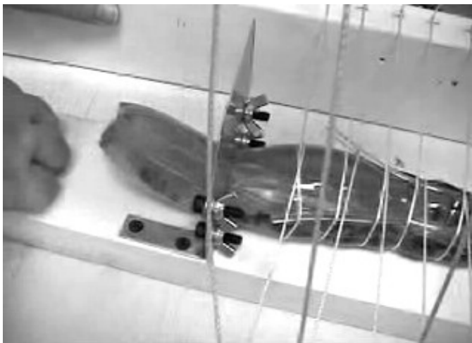
FIGURE 10: Moving through a hole with a diameter smaller than half of its nominal width.
