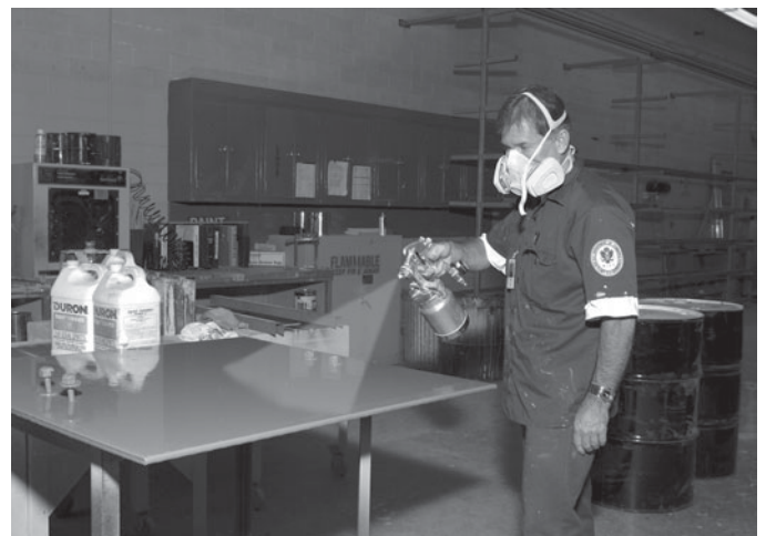
Spraying machine operators use spray guns to coat a variety of products and surfaces.
