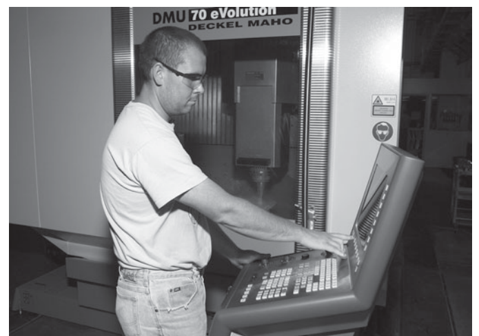
Using specialized control modules, computer control programmers and operators make adjustments to the machining process.
