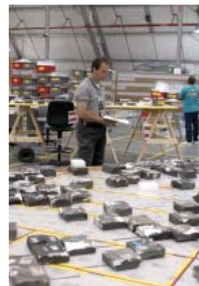
United Space Alliance technician Woody Woodworth identifies pieces of Thermal Protection System tile from the left wing of Columbia recovered during the search efforts in East Texas.
