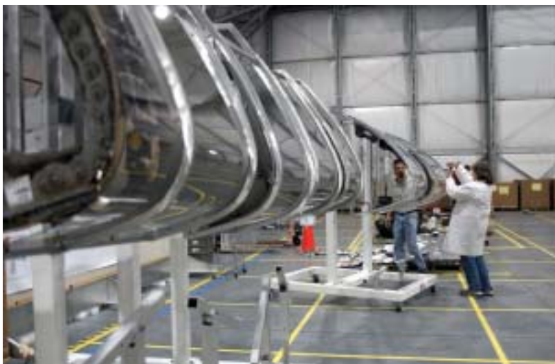
Members of the Columbia Reconstruction Project Team seek to place a piece of debris from Columbia on this replica of the leading edge of the left wing.
